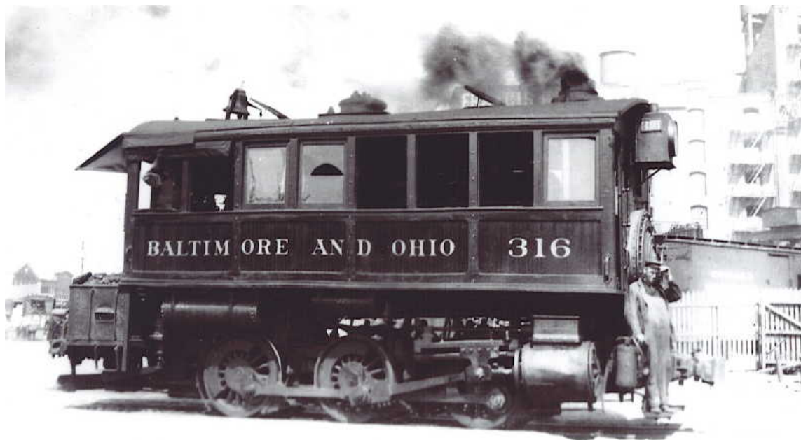
B&O #316 at West 26th Street, New York City in 1922. The rods are grimy now but the monel cylinder jackets still on it hint of a spiffier day. Photographer unknown, collection of the Baltimore & Ohio RR Historical Society.
