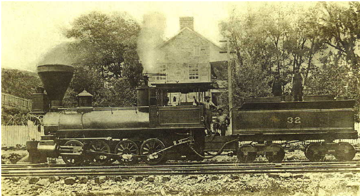
B&O #32, a Perkins designed eight-wheel coupled freight engine built in July 1865 at Mount Clare; stands ready at Weverton, MD in 1871.
